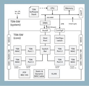
Schematic diagram of the TSN-SW IP Core.
