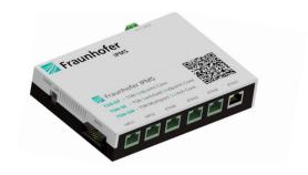
TSN Evaluation Kit: Xilinx ZCU102 or Intel Netleap (Cyclone V SoC); implemented IPMS TSN-IP core for endpoint applications (TSN-EP).
