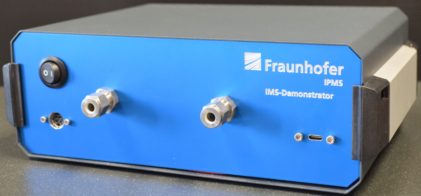
Figure 1: Demonstrator setup with integrated IMS chip module
