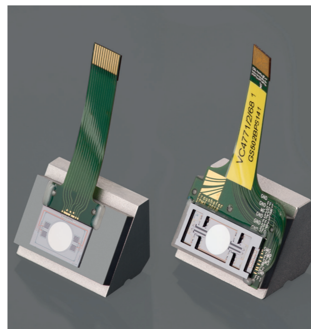
▲ 1D MEMS scanner, identical aperture 5 mm left: 1D resonant, right: 1D quasi-static
