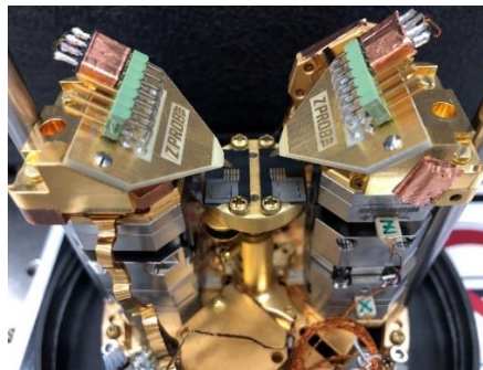
Realised first interposer mounted into the cryogenic test setup. © Fraunhofer IPMS
