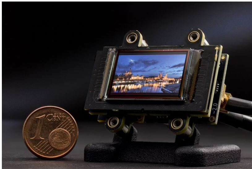
Figure 1: Universal Data Converter for Display Data (UDDC) with high-resolution OLED microdisplay (WUXGA) ©Fraunhofer IPMS, Photographer: Sebastian Lassak
