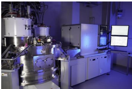
The cryogenic on-wafer prober at Fraunhofer IAF enables fully automatic characterizations of up to 25 whole 200-mm or 300-mm wafers with devices for quantum technologies. © Fraunhofer IAF
