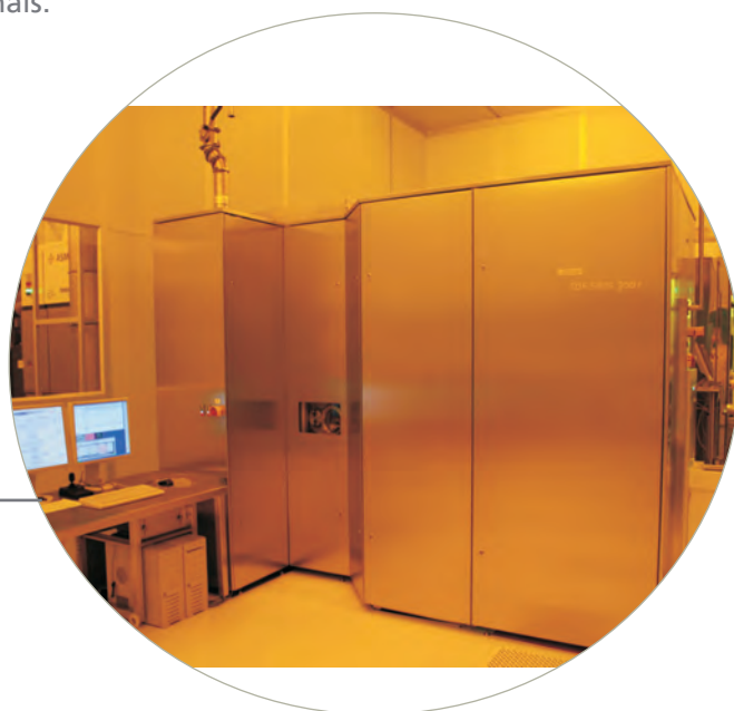
Abb. 5 fig. 5 Das TOF-SIMS Tool des Fraunhofer CNT The TOF-SIMS tool of the Fraunhofer CNT
