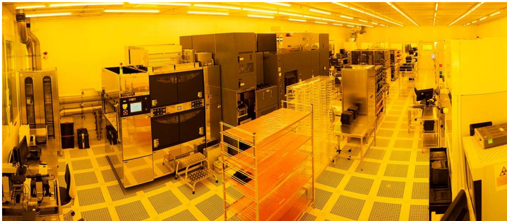
MEMS-Lithography-Capabilities with 248 nm DUV-Cluster and 365 nm iLine Stepper. ©Fraunhofer IPMS
