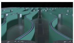
Animation of a MEMS micro loudspeaker device with actuator pairs arranged in parallel. © Fraunhofer IPMS
