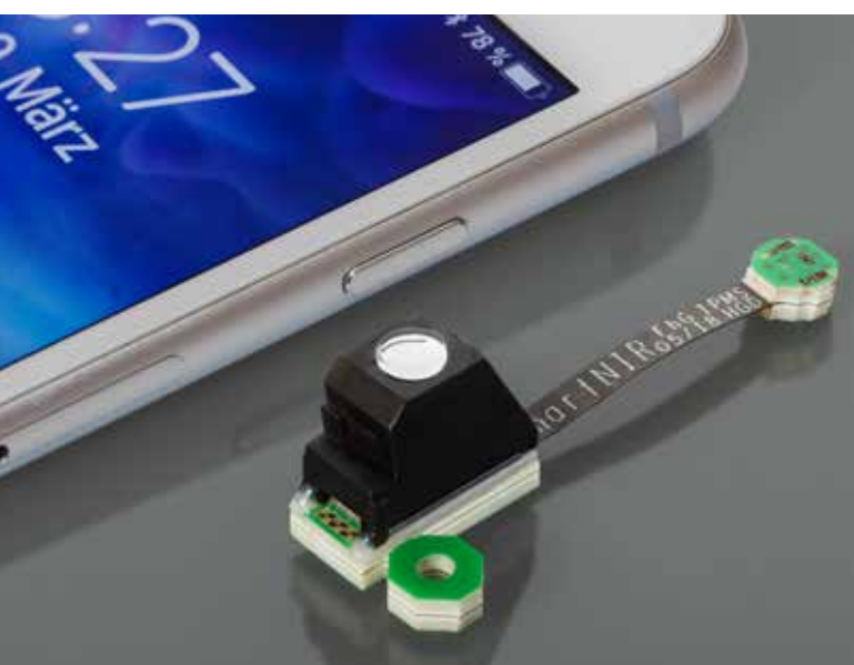
Miniaturized NIR spectrometer developed by Fraunhofer IPMS
