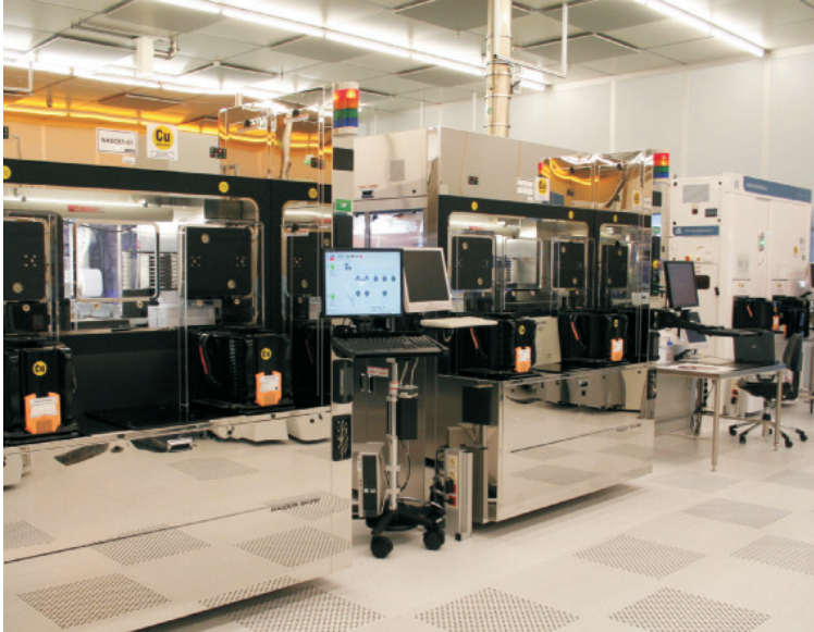
▲ CNT cleanroom with ULK, copper plating CMP tools.
