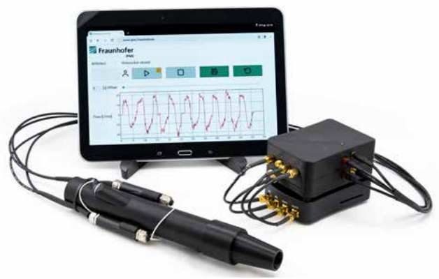
Figure 2: Ultrasound spirometer by Fraunhofer IPMS
