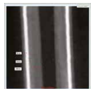
Dark field image of the MIM stack on the side wall of the trench: the \text{HfO}_2 layer is imaged as a bright layer as it contains the heaviest atoms
