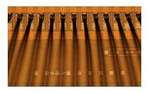
Fan-out test chip for electro-optical conversion.
